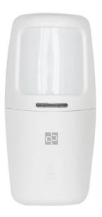
The battery powered wireless motion sensor is designed to detect the movement of a person in a guarded room. The PIR sensor uses the technology of digital infrared control with flexible logic and intelligent analysis algorithms, which allows distinguishing signals of interference from human body signals.
