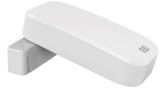
The battery powered wireless door/window sensor is designed to detect the opening of doors, windows, hatches, gates. The sensor consists of a magnet and a sensor (reed switch), which determines the change in the magnetic field. When the magnet moves away from the sensor, the detector detects the change and sends a signal to the device to which it is connected.
